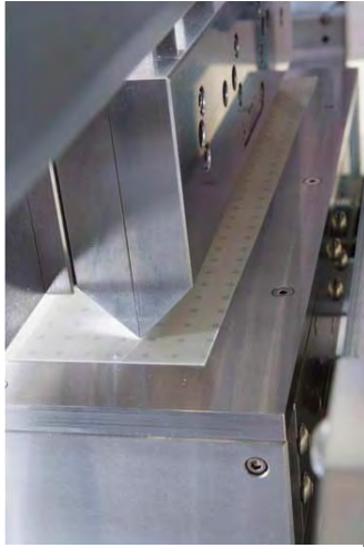
Liberty slot die in patch coating system
