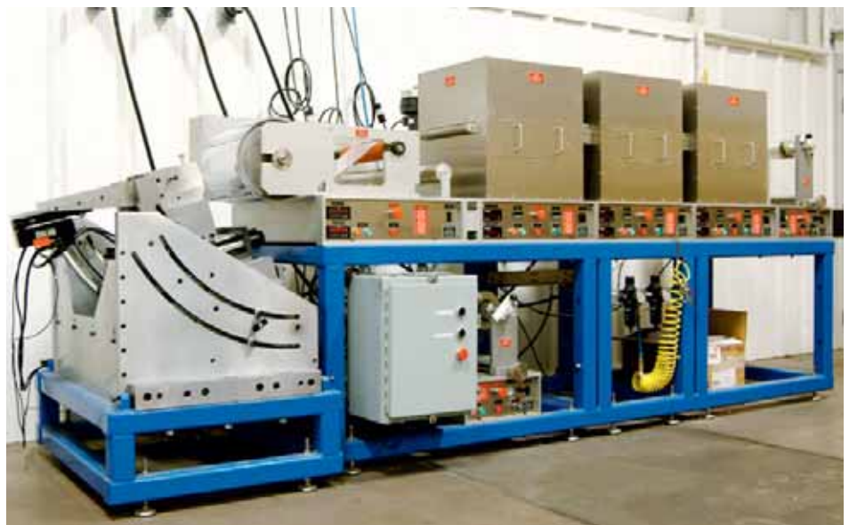
PROCESS LABS FOR RENT: NEW EDI SERVICE. This slot die coating system is one of three laboratories that EDI has installed in its new Technology Center. The others are for cast film and extrusion coating/laminating, respectively. Instead of tying up their own full-scale production lines with trial runs, companies can rent these facilities and use them under protection of a confidentiality agreement with EDI.
